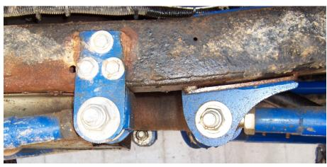
Mount the upper links into the Frame Bracket. The order is bolt, washer, bracket, spacer, rod end, spacer, washer, thin nut.
