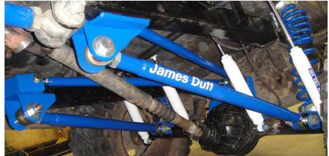
Thread the Jam nuts and Rod Ends into the proper Left Hand or Right Hand adapter in the upper link bars. Do not tighten all the way. Be sure to leave space so the Rod End can be adjusted both ways. So when measuring placement of the frame bracket the Rod end will have adjustability both directions.
