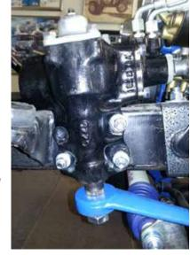
tightening any of them. Finish with another 1/2" washers and 1/2" NC Nyloc nut on each. Torque to 60-80 ft lbs. Note: This box has 4 bolt holes. After tightening the three bolts, you can drill the 4th hole through the frame using the box as a template and install the fourth 1/2"-13 x 4 1/2" GR5 bolts with 1/2" washers at this time with the same torque specs.
